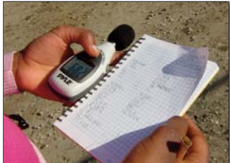
Collecting data on noise levels at Baldwin Hills Scenic Overlook State Park with a sound level meter
